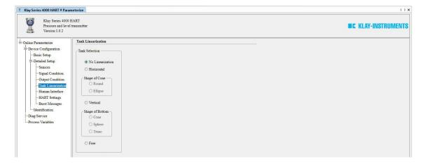
With the option **Free**, a linearization can be configured up to 70 points. For each linearization point a line must be added in the table as shown below. To add a linearization point, select the line where a new linearization point must be added as shown below. The **X-Axis** value must always be filled with a
