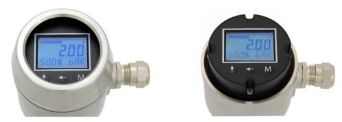
Unscrew the cover to get access to the push buttons of the display. The display can be turned max. 180° to put it in the desired position for reading. The complete display unit can be taken out to be able to adjust the transmitter. Be careful when taking out the display as the length of the wiring is limited. Please ensure that the cover is fastened properly after adjusting the display to ensure the sealing of the housing.
