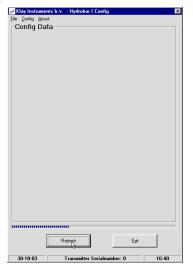
The software will automatically search for the HydroCER-I that is connected (can take a few seconds). When the transmitter is not found you have to choose another COM-port. With Config (Com settings) you can do this (see window below).
