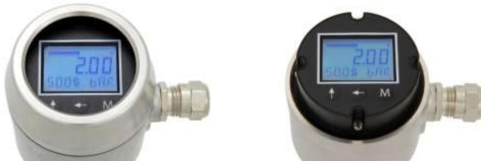
Unscrew the cover to get access to the push buttons of the display. The display can be turned max. 180° to put it in the desired position for reading. The complete display unit can be taken out to be able to adjust the transmitter. Be careful when taking out the display as the length of the wiring is limited. Please ensure that the cover is fastened properly after adjusting the display to ensure the sealing of the housing.
